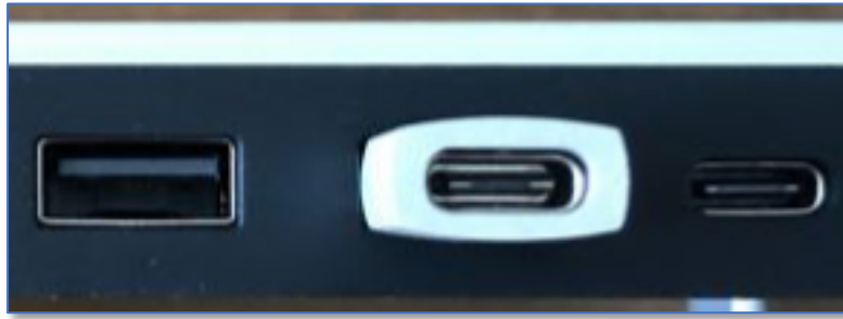
Adapter Plugged Into a USB-A Port (Result: Converts a USB-A Port to a USB-C Port)
