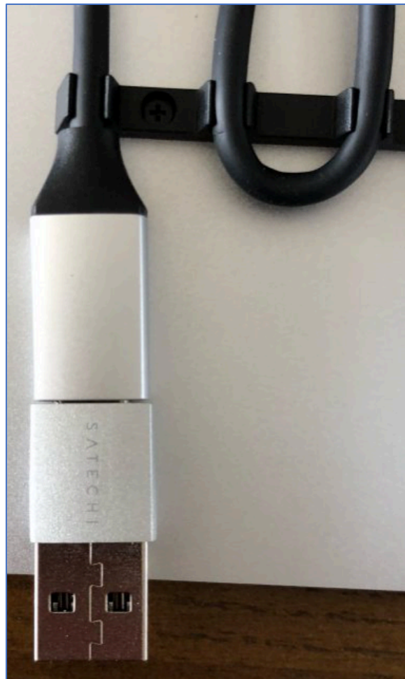
Adapter Connected to the Cable (Result: USB-A Connector for an Older iMac)
